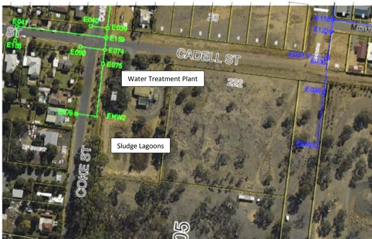
Figure 9- Aerial Photograph of Hay Water Treatment Plant showing location of potential pollutants on site and surrounding stormwater drainage structures. The Green and blue lines represent the piped stormwater drainage system. Given the existing drainage system within the site it is very unlikely that any spilled chemicals would reach the external stormwater system.
